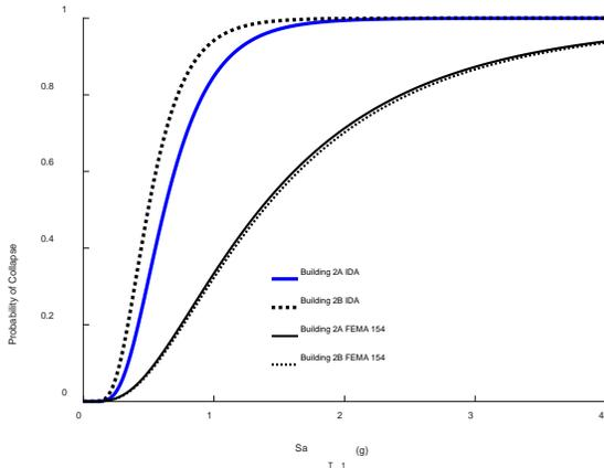
Figure 8 Collapse fragility curves from incremental dynamic analysis (including *SSF* and *MU*) and FEMA 154 checklist for Buildings 2A and 2B
