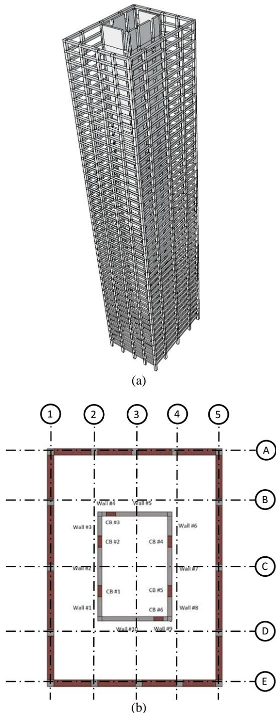
Figure 1 (a) Isometric view and (b) plan layout of dual moment frame system
