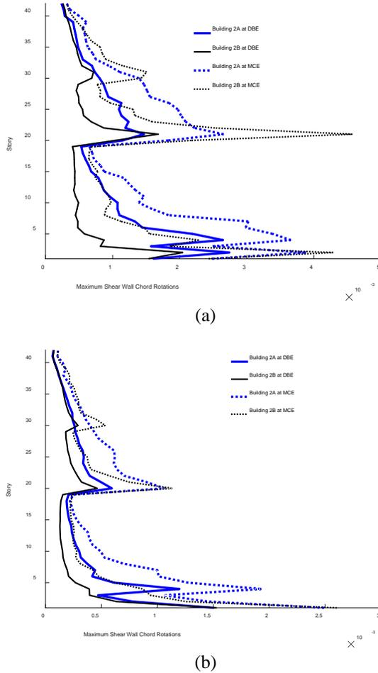
Figure 6 Median of maximum chord rotation profile in shear walls (a) 5 (X-Direction) and (b) 7 (Z-Direction)
