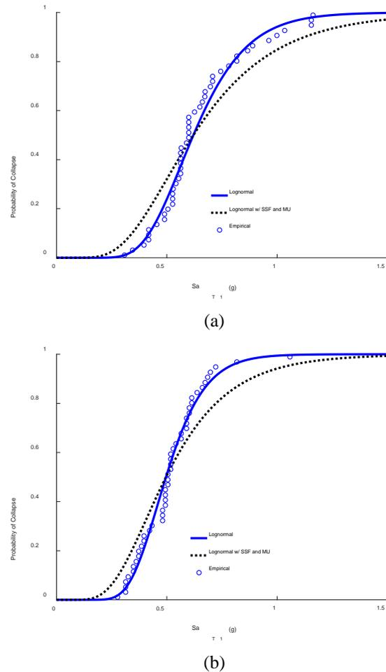
Figure 7 Collapse fragility curves from incremental dynamic analysis including the effects of spectral shape factor (*SSF*) and modeling uncertainty (*MU*) for (a) Building 2A and (b) Building 2B
